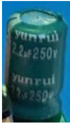
Electrolytic capacitor 2.2uF.250V .105 °C
