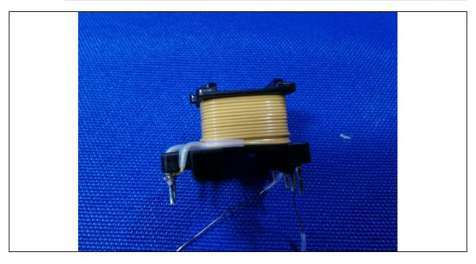
Details of: Fig 12. Transformer SR-JB1002-12W (For circuit diagram B models)
