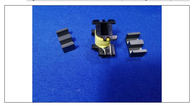
Details of: Fig 14. Primary winding Transformer SR-JB1002-12W (For circuit diagram B models)
