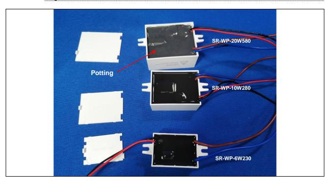
Details of: Fig 4. Internal view before potting
