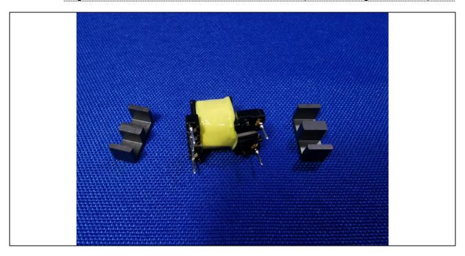
Details of: Fig 18. Primary winding Transformer for SR-JB1001-6W (For circuit diagram A models)
