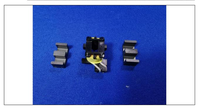
Details of: Fig 10. Primary winding view Transformer SR-JB1003-20W (For circuit diagram C models)
